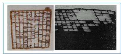
Observe how the grid plate lead material is dissolved as a result of corrosion effects. As the grid plate dissolves the grid plate cannot hold the lead paste mass. This failure then causes that active material paste falls out of the surface grid plate. Less lead paste means less active material to produce energy.
